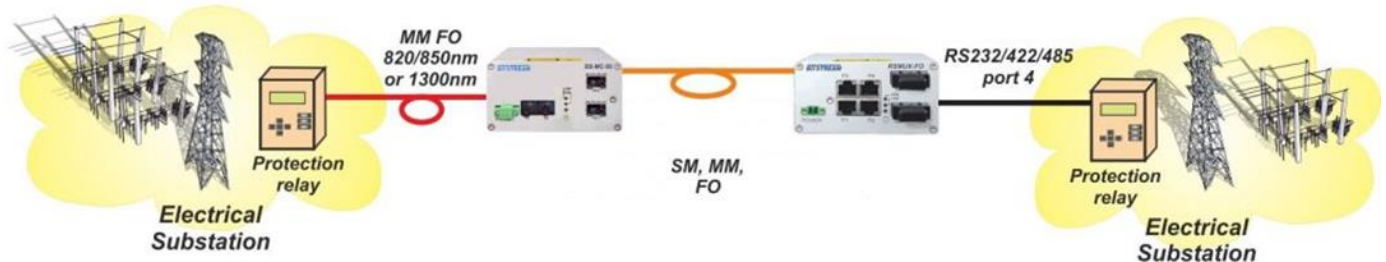
Fig. 2. Example application of cooperation with RSMUX3-FO multiplexer.
